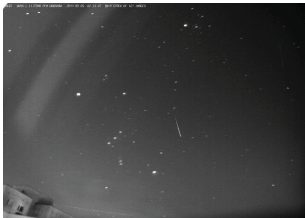
Figure 2 – Image from the QHY5-LII Mono camera with Tamron 3-8mm f/1.0 megapixel lens. A meteor is visible in the middle part of the image. Clear weather and a moonless night with significant light pollution.
