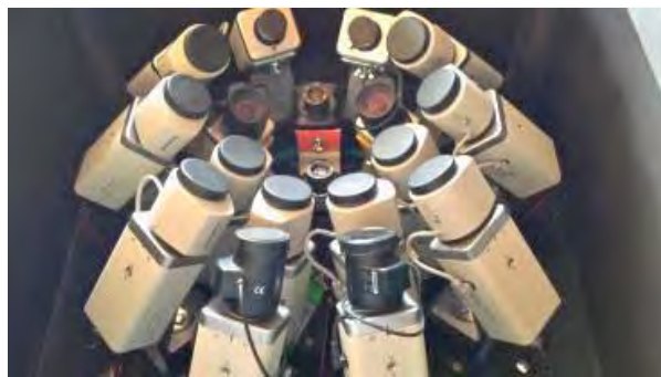
Figure 9 – 18-camera amateur array at the Foresthill, CA single-CAM station.
