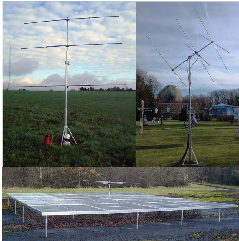
Figure 2 – Images of BRAMS antenna systems directly managed by BISA (Top left: Yagi at Humain Radio Astronomy Station. Top right: Crossed Yagi at BISA facilities, Uccle. Bottom: Turnstile at Dourbes Geophysical Center).
