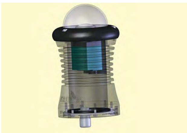
Figure 5 – FRIPON housing with passive-cooling. The main body is semi-transparent to show the camera. The overall dimensions are 150 x 70 mm and the weight is less than 1kg.
