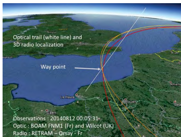
Figure 11 – 3D Interception of 3 ellipsoids (cut @ altitude 95 km) and optical trail calculated by BOAM (white line).
