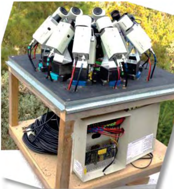
Figure 10 – Inside view of the 18-camera setup, showing cameras, brackets, and 16-port power supply.
