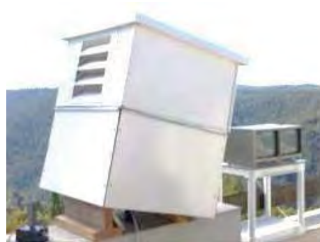
Figure 15 – 18-camera box housing. Ventilation maintains internal temperature close to ambient.
