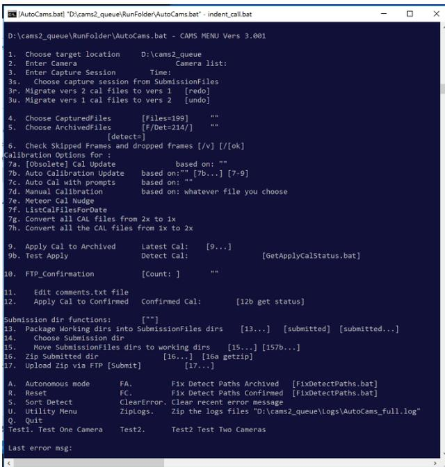
Fig 8. Screenshot of AutoCAMS.bat checklist menu. Notice how steps 1-17 are in the order they should be performed. Detection is actually #45 on the utility menu, since at that time we were using real-time detection.
