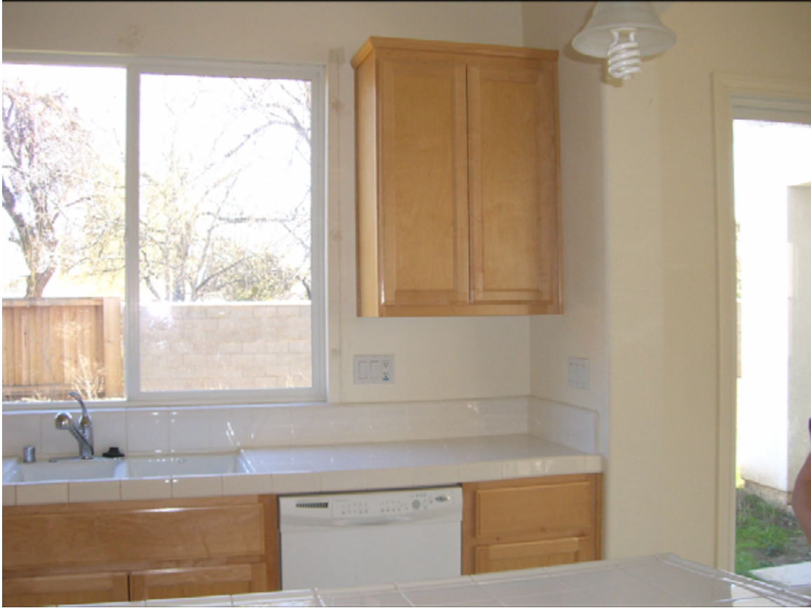
Under-cabinet dual sink. Sink is porcelain-covered cast iron sink. 1/2 horsepower insinkerator. Five cycle, Whirlpool Quiet Partner III dishwasher.
